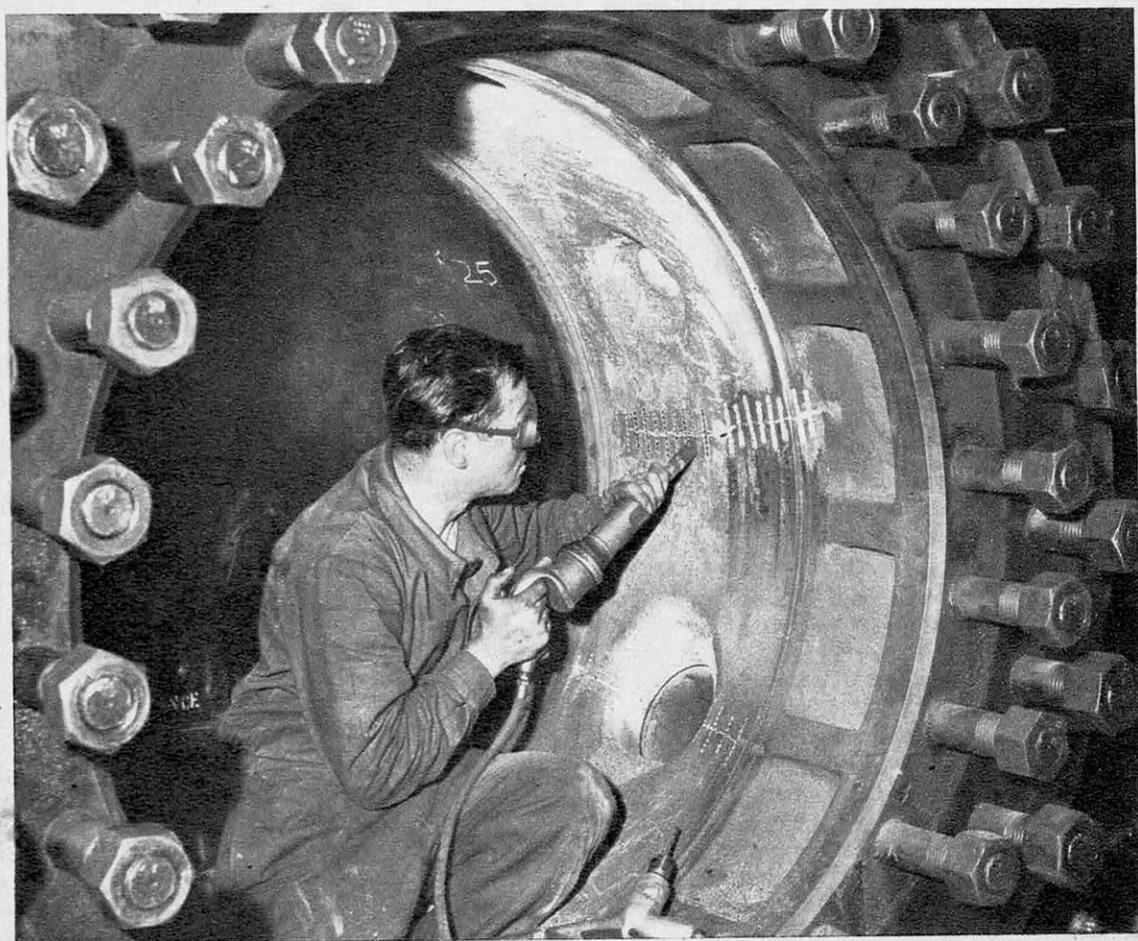
EN TRAVERS DE LA FENTE ON CREUSE DES LOGEMENTS OÙ ENFONCER DES BARRETTES
