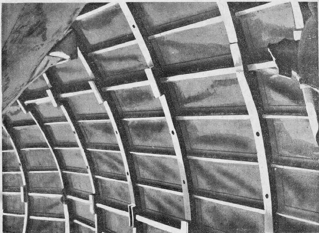
FIG. 5. — LA CHARPENTE DE LA V-2 AU NIVEAU DU COMPARTIMENT DES RÉSERVOIRS
