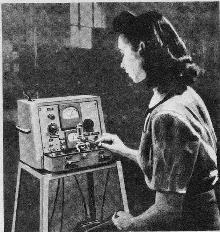
FIG. 4. — LE DÉTECTEUR DE FUITES DANS SA RÉALISATION INDUSTRIELLE
