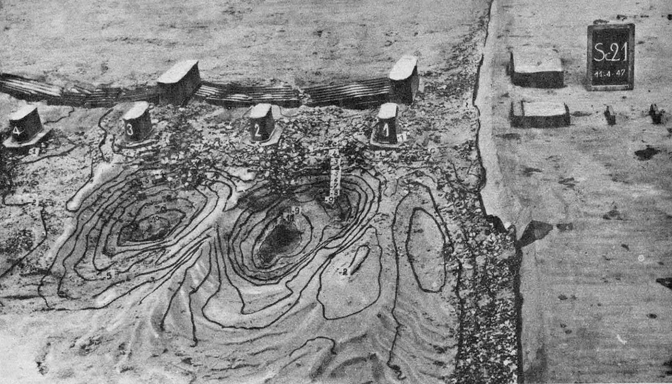
FIG. 14. — ÉTUDE SUR MODÈLE RÉDUIT DE LA PROTECTION, CONTRE LES AFFOUILLEMENTS, DES PILES DU VIADUC DE SAINT-CLAIR SUR LE RHONE, A LYON
