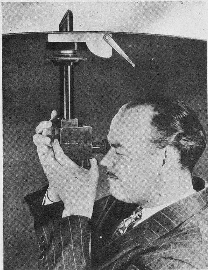
FIG. 2. — LE SEXTANT PÉRISCOPIQUE PERMETTANT DE FAIRE LE POINT DANS UN AVION A CABINE ÉTANCHE VOLANT A HAUTE ALTITUDE (KOLLSMAN INSTRUMENT DIVISION)
