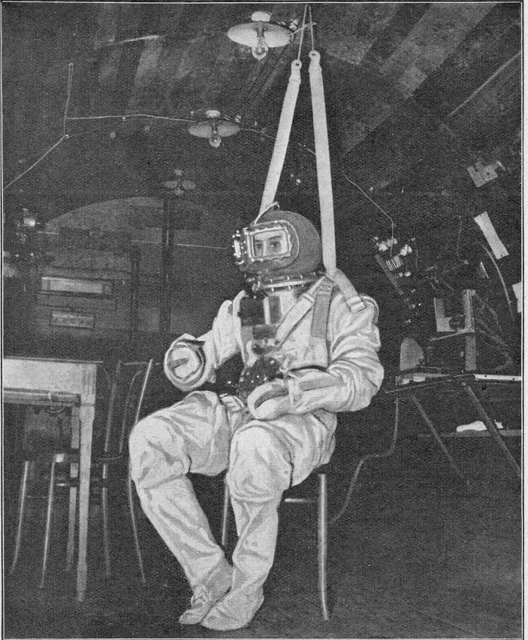
LE SCAPHANDRE STRATOSPHERIQUE DES DOCTEURS ROSENSTIEL ET GARSAX, EN ESSAI DANS LE CAISSON PNEUMATIQUE DU BOURGET, PRÈS PARIS
