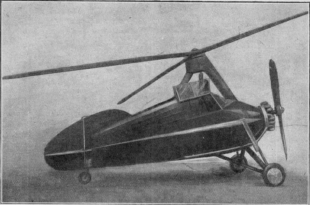
FIG. 2. — LE NOUVEAU TYPE D'AUTOGIRE, AVEC LEQUEL S'EST PRODUIT L'ACCIDENT, NE COMPORTE PLUS DE PLAN FIXE
