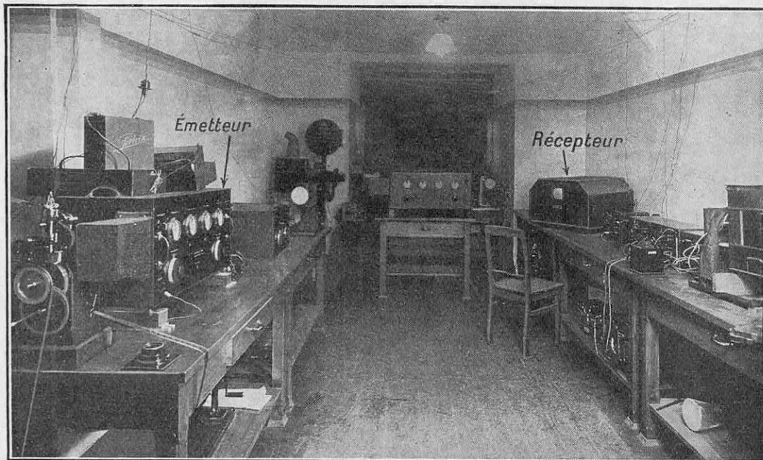
FIG. 6. — DANS LE LABORATOIRE DE MANFRED VON ARDENNE : A GAUCHE, L'ÉMETTEUR, ET, A DROITE, LE RÉCEPTEUR DE TÉLÉVISION PAR RAYONS CATHODIQUES
