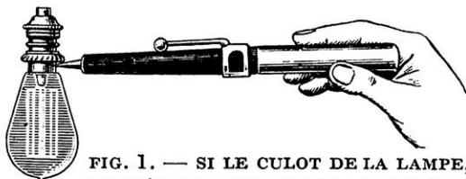
FIG. 1. — SI LE CULOT DE LA LAMPE, QUE L'ON TOUCHE AVEC LA POINTE DE L'APPAREIL, EST SOUS TENSION, UN VOYANT APPARAÎT IMMÉDIATEMENT
