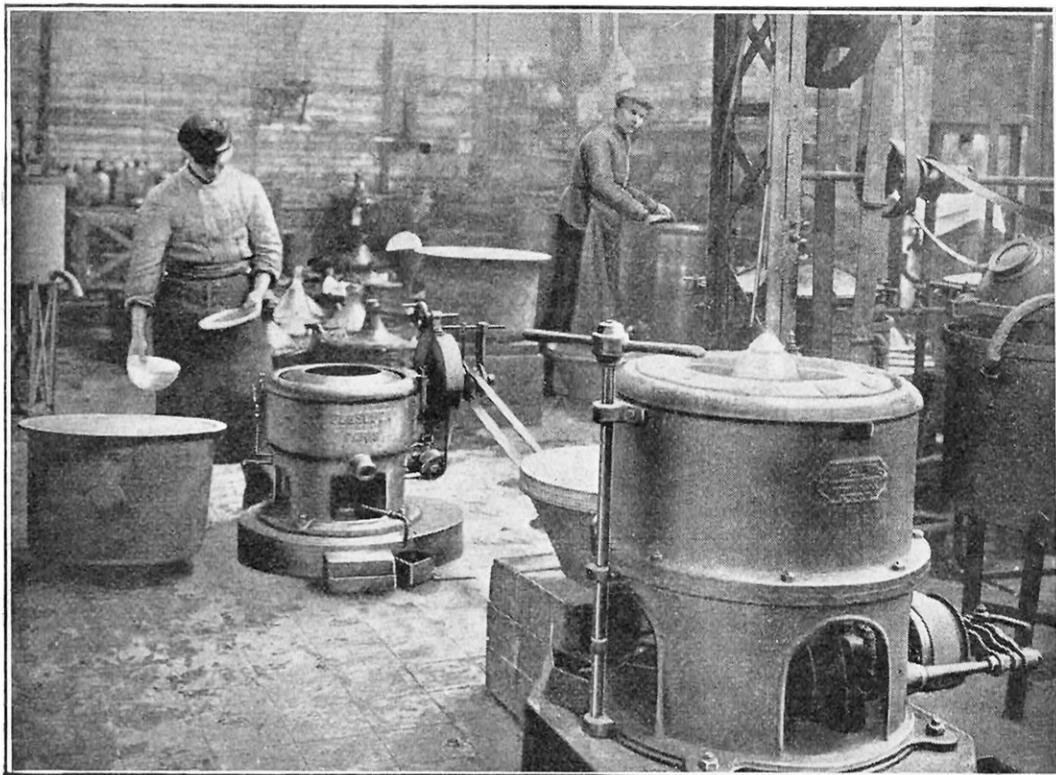
APRÈS LE BENZOYLAGE ET LA CRISTALLISATION DANS L'ALCOOL, LA STOVAÏNE EST ESSORÉE A LA TURBINE, PUIS SÉCHÉE A L'ÉTUVE ET TAMISÉE
